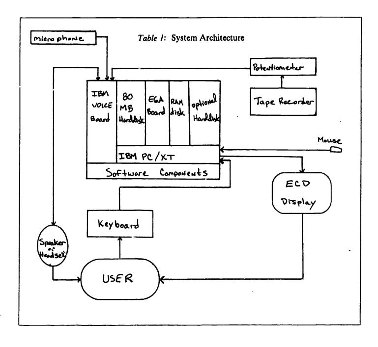
Table 1, above shows in graphical form, the system architecture which contains various hardware components and the software component. The next section provides in greater detail the actual hardware devices needed to implement this project and the remainder of the system design will provide the details of the software component, shown above as one block.
